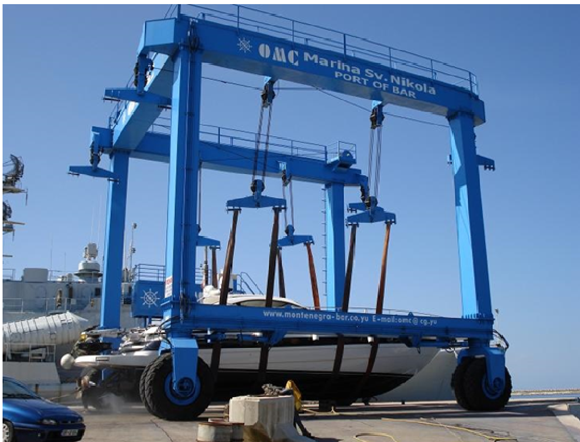
Slika 8. Portalna dizalica (travel lift) Ascom ATS 260, Marina OMC, Bar, 2017. 52
